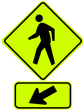
Figure 55: W11-2 sign with W16-7L left diagonal arrow
